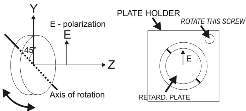
The alignment for **half-wave retardation** is achieved when the plate is positioned between two **parallel** polarizers and by tilting the plate the transmitted light is totally **extinguished**. In order to rotate the polarisation plane by an arbitrary angle, use the rotation part with degree dialing.
