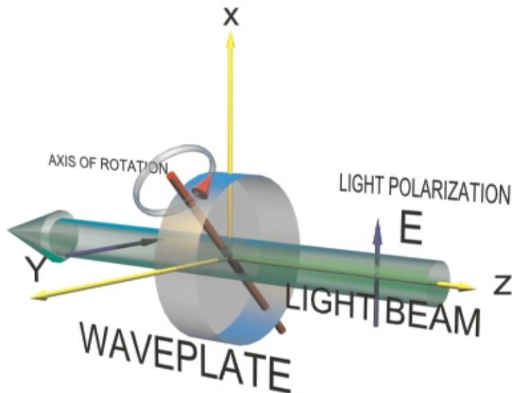
The required phase retardation is achieved by tilting the plates by  $8^\circ - 15^\circ$ . This design is aimed at avoiding light reflection back to the laser system which in many cases results in complications.
