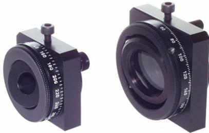
2. Rotate the screw until the retardation plate is parallel to the plane of the holder. After that align the whole device so that both plate and the holder are perpendicular to the incident beam. The light beam will be then reflected from the waveplate exactly in the backward direction.
