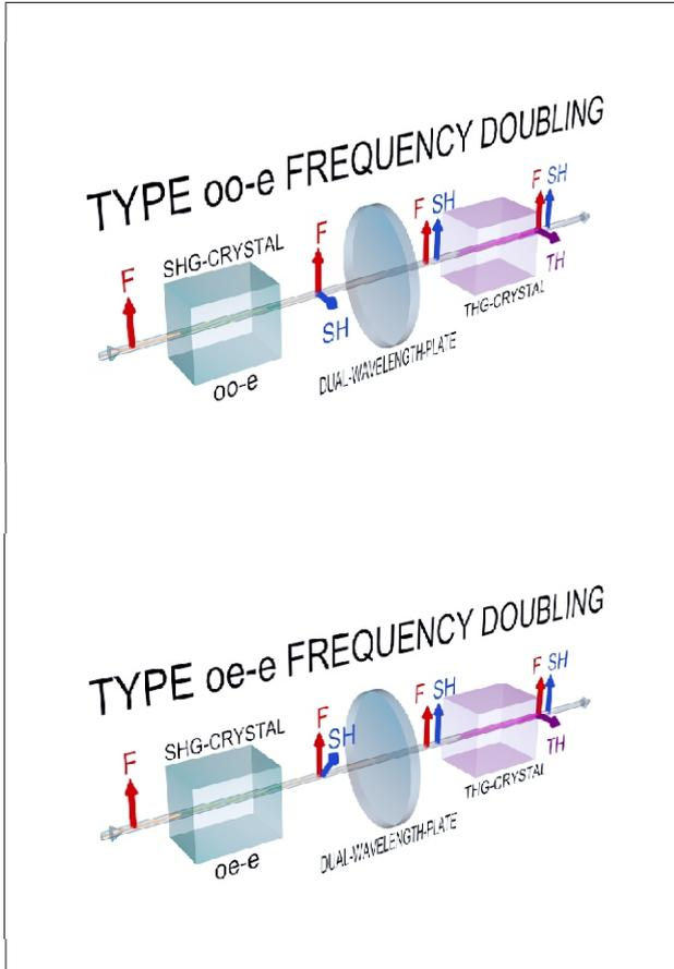
Efficient frequency-tripling of laser light requires rotation of the polarization plane of the fundamental F or the second harmonic SH after the frequency doubling crystal in order to make the planes parallel for efficient interaction in the frequency tripling crystal.
