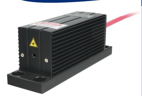
wide range of passively Q-switched lasers with pulse durations below 1 ns and extremely high peak powers at 1064 nm with excellent TEM<sub>00</sub> beam profile are offered by ALPHALAS. The PULSELAS®-P lasers feature proprietary microchip design. The monolithic laser cavity is permanently aligned and therefore extremely stable.
